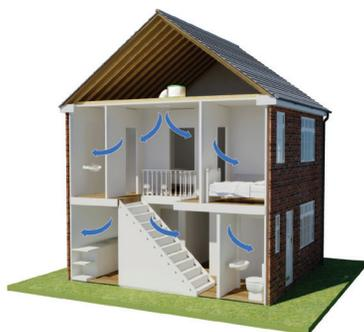
Our PIV systems are accredited with BBA certification and also comply with building regulations. The EnviroVent units are sophisticated whole house ventilation and condensation control units. By drawing in fresh, filtered and clean air from outside, they gently ventilate the home from a central position on a landing in a house or the central hallway in a flat or bungalow.
