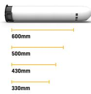
The heatSava is available in two cell diameters: 100mm for bathrooms and WC's and the 150mm for kitchens, ideal for both refurbishment and new build installations. Fitting neatly into almost any wall depth, the length of the cell is available to suit external wall depths of up to 330mm, 430mm, 500mm and 600mm.
