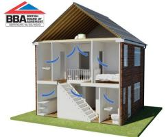
The system works particularly well with Mechanical Extract Ventilation (MEV) and can also be used with Envirovent high quality Intermittent Extract Fans. The use of PIV can also negate the requirements for unsightly, draughty trickle vents in windows.
