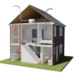
This constant supply of clean, tempered air into the property creates a healthy, filtered environment maintaining stable humidity levels, free from condensation and mould.
