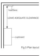
O Clearance - Ceilings First measure the wall depth. If installing into a new build application, we recommend that the unit should be installed in the position below (option 1). If installing into an existing wall sleeve which is located near to the ceiling, the heatSava can be installed horizontally or vertically (options 2-4).
