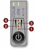
In terms of maintenance, the DataSync technology makes it easier for you. The monitors signal the appropriate moment to change the bag or empty the canister of your vacuum unit, and even indicate when mechanical maintenance is recommended. All this information is available on the front of the unit, as well as on the hose handle, right at your fingertips!
