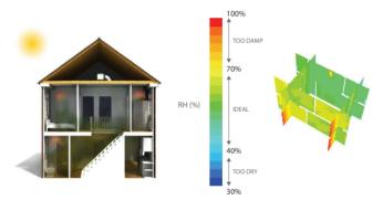
Humidity is diluted, displaced and replaced. Relative humidity is still between 55-65%
